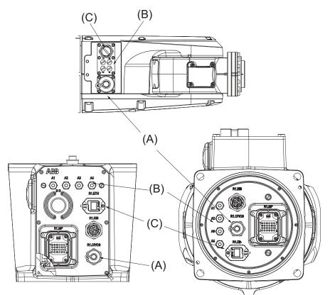
Hose for compressed air is also integrated into the manipulator. There are 4 inlets at the base (R1/8") and 4 outlets (M5) on the tubular housing.
