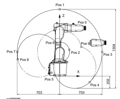
IRB 1200-7/0.7 Working range, positions at wrist center and angle of axes 2 and 3 The illustration shows the unrestricted working range of the robot.
